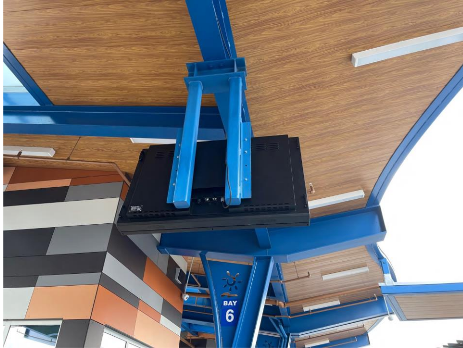
Figure 5: NANOV 55" Outdoor Single-Sided Real-Time Passenger Information Digital Sign with Ceiling Mount in Lauderhill Bus Bay – Back View
