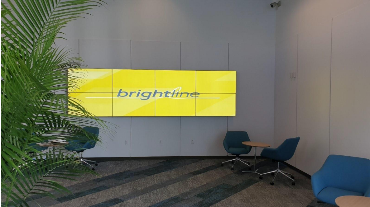
Figure 3: NANO V 2X4 Videowall – Select Lounge Area 1.8mm Super Narrow Bezels with 46" Full HD Displays
