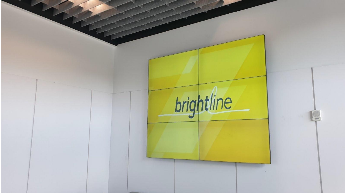
Figure 5: NANOV 3X2 Videowall – Wall in Smart Lounge 1.8mm Super Narrow Bezels with 55" Full HD Displays
