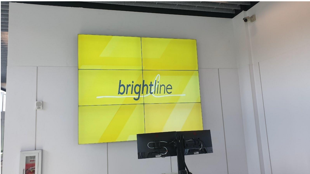
Figure 4: NANO V 3X2 Videowall – Wall Behind Security Checkpoint 1.8mm Super Narrow Bezels with 55" Full HD Displays
