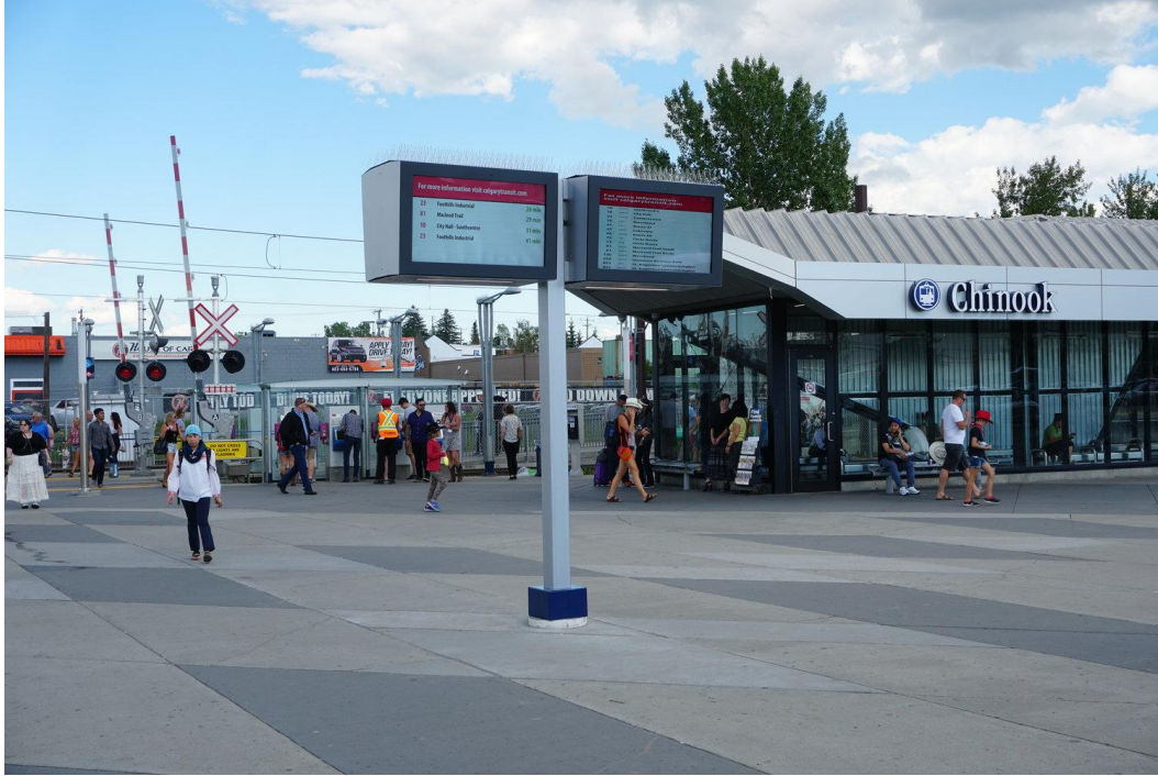
Figure 3: Two of NANOV's 55" Single-Sided Passenger Information Display Signs (PIDS) attached to pole via side mounts at Chinook CTrain Station in Calgary, Alberta
