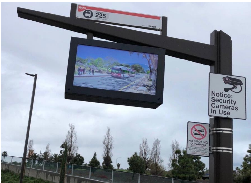
Figure 4: NANOV 46" Double-Sided Real Time Variable Message Sign (VMS) in San Diego Rapid Bus Service Station
